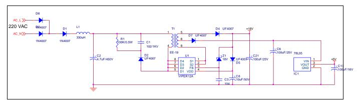
Figure 2-2 Power Supply Circuit
